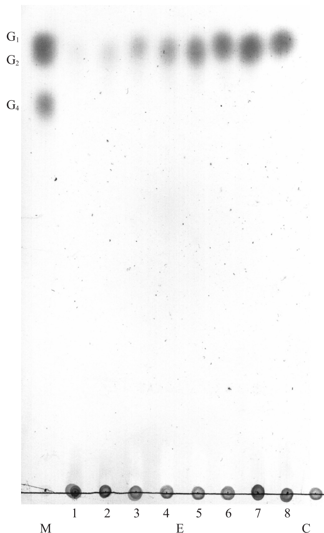
Figure 5. TLC chromatogram of hydrolysis products of mutan obtained with mutanase preparation from T. harzianum . Hydrolysis conditions as in Materials and Methods. The samples applied were: M – marker, G 1 – glucose, G 2 – nigerose, G 4 – nigerotetraose; E – sample from enzymic digestion of mutan at different periods of incubation: 1 (30 min), 2 (1 h), 3 (2 h), 4 (3 h), 5 (6 h), 6 (12 h), 7 (24 h), 8 (48 h); C – heat-inactivated enzyme. Four microliters of each sample were spotted on the TLC plate. The locator was naphthylethylenediamine dihydrochloride reagent. See the text for the other experimental details.
