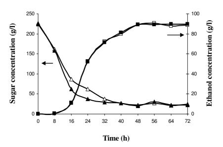
Figure 5. Batch fermentations using ALM carriers with dimensions of 9 x 9 x 3 mm<sup>3</sup> (open symbols) and 20 x 20 x 3 mm<sup>3</sup> (filled symbols);  $\Delta$ ,  $\blacktriangle$  = sugar:  $\Box$ ,  $\blacksquare$  = ethanol.
