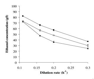
**Figure 6.** Ethanol concentration at dilution rates of 0.1-0.3 h<sup>-1</sup> and initial sugar concentrations of 200 g/L ( $\Box$ ), 220 g/L ( $\blacksquare$ ), and 248 g/L ( $\blacktriangle$ ).
