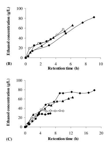
**Figure 8.** The steady-state ethanol concentration profiles at initial sugar concentrations of 200 g/L (A), 220 g/L (B), and 248 g/L (C) and at superficial velocities of 4.8 cm/h ( $\blacklozenge$ ), 6.9 cm/h ( $\bigstar$ ), 8.7 cm/h ( $\circ$ ), and 13.0 cm/h ( $\bullet$ ).
