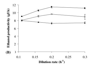
**Figure 7.** Ethanol productivity at dilution rates of 0.1-0.3 h<sup>-1</sup> and initial sugar concentrations of 200 g/L ( $\Box$ ), 220 g/L ( $\blacksquare$ ), and 248 g/L ( $\blacktriangle$ ).
