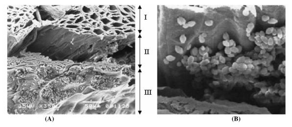
**Figure 2.** (A) Cross-section of the ALM after 72 h of ethanol fermentation. The ALM consisted of loofa fiber (I), a hollow space between the loofa fiber and alginate gel (II), and alginate gel (III). (B) A higher-magnification view of the hollow space.
