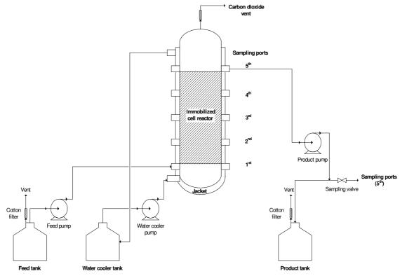
Figure 1. Schematic diagram of the immobilized-cell PBR.
