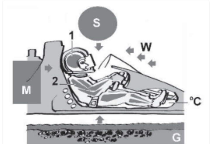
Fig. 1 – Diagram of the cockpit environment during race – External sources of heat: S, solar; M, mechanical; G, ground; W, air mass. Internal sources of heat: 1, brain metabolism; 2, muscular physical activity.
