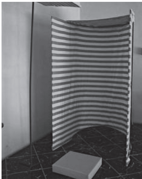
Figure 1. Foam-Laser Dynamic Posturography cabin proposed by Castagno (1994).
