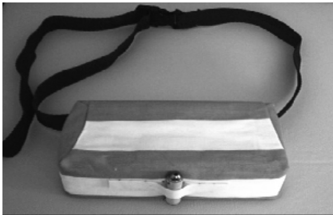
Figure 2. Belt made with nylon and foam fabric, with attachment on the ends adjustable to the participant's waist level, with attached laser beam pen.
