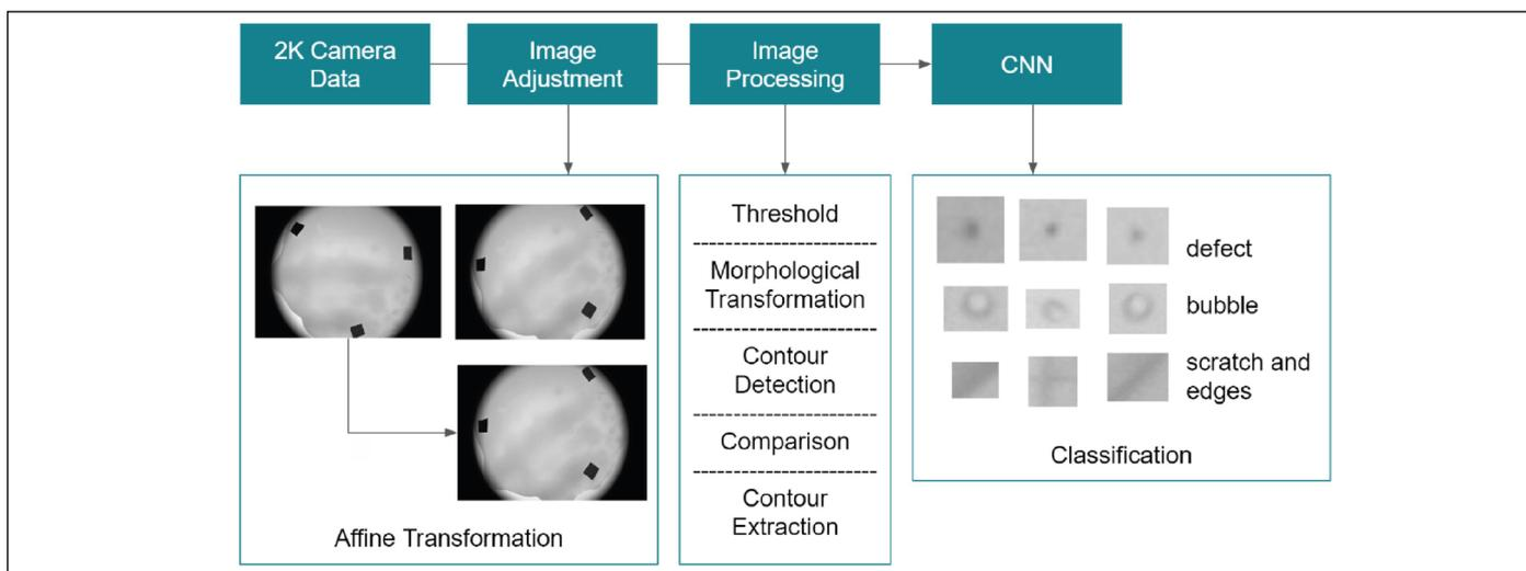
Figure 1. Contour extraction algorithm for image damage location.
