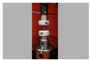
Figure 2. A graft fixed to the testing machine showing the wooden tubes and containing belts.
