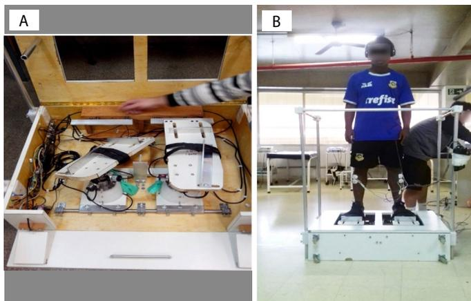
**Figure 1.** A. Sudden inversion platform with foot support and lateral support. B. Positioning the subject on the platform.
