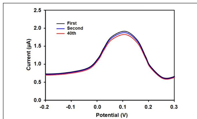
**Figure 3.** Stability effects of the  $\text{Fe}_2\text{O}_3\text{-NiO}@\text{GO}/\text{GCE}$  reaction to the 20ng/l erythropoietin into 0.1M PBS at 10 mV/s scan rate, with the first, second, and 40th DPV responses.
