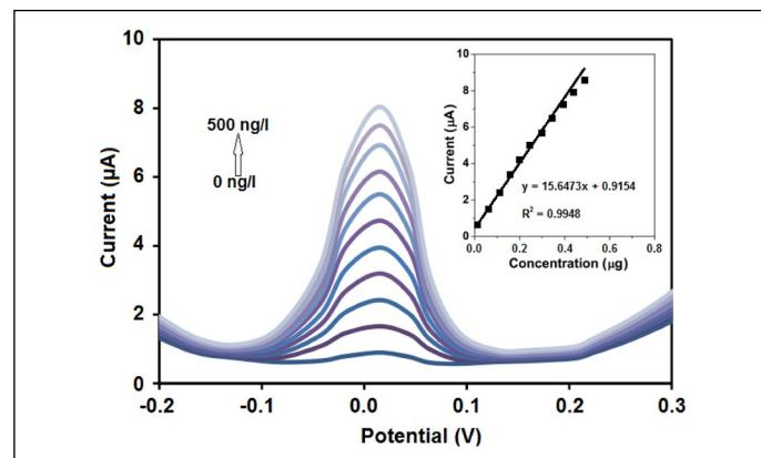
**Figure 4.** DPV and calibration curves of electrodes to add different level of protein into 0.1M PBS at 10 mV/s scan rate.
