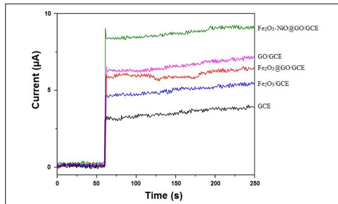
**Figure 2.** Amperometric of GCE, GO/GCE, Fe<sub>2</sub>O<sub>3</sub>/GCE, Fe<sub>2</sub>O<sub>3</sub>@GO/GCE and Fe<sub>2</sub>O<sub>3</sub>-NiO@GO/GCE with adding 50µM DA into 0.1M PBS.
