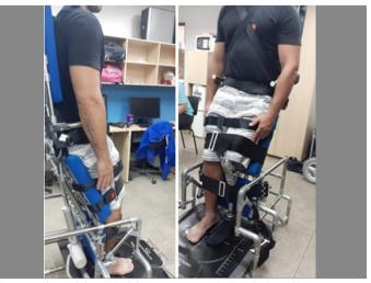
Figure 2. Elevated device. Stabilization straps on the hip, thigh, and leg region.
