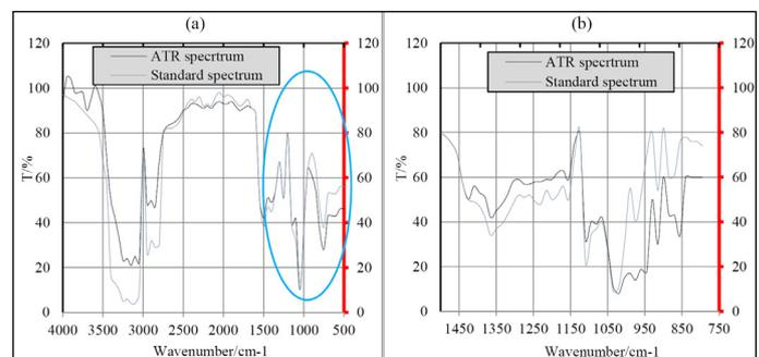
**Figure 3.** Comparison diagram of glycerol spectrum measured by optical fiber infrared spectral imaging technology probe measuring device and standard glycerol spectrum. ((a) Comparison diagram of the two spectra at full band (b) Comparison diagram of the spectra in the elliptical region after amplification)
