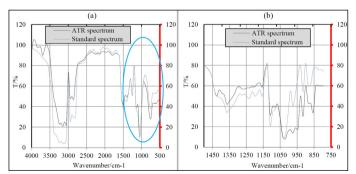
**Figure 3.** Comparison diagram of glycerol spectrum measured by optical fiber infrared spectrum imaging technology probe measuring device and standard glycerol spectrum. ((a) Comparison diagram of the two spectra at full band (b) Comparison diagram of the spectra in the elliptical region after amplification)
