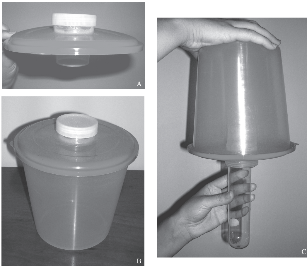
Fig 1 SECTAB storage system for tabanids. A) Horizontal view of large cover showing the smaller flask inside it, B) Complete view of the device, C) Coupling of the SECTAB device and the collecting tube.
