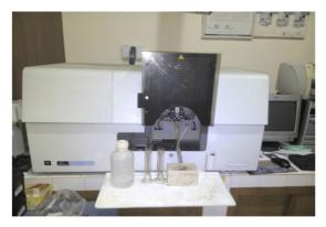
Figure 3. Atomic absorption spectrophotometer used for the analysis of heavy metals i.e zinc, lead, chromium and nickel present in the extracted tissues of muscles and gills.
