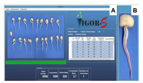
**Figure 2.** Screen of the Vigor-S<sup>®</sup> analysis system software with a cowpea sample (BRS Tumucumaque) two days after sowing the germination test (A); seedling detail identifying the primary root (red) and the hypocotyl (blue) (B).
