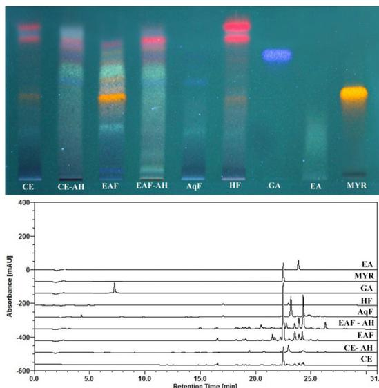
**Figure 1.** TLC and HPLC profiles obtained for crude extracts and fractions from leaves of *E. uniflora*. CE, Crude Extract; CE-AH, Crude Extract After Hydrolysis; EAF, Ethyl Acetate Fraction; EAF-AH, Ethyl Acetate Fraction After Hydrolysis; AqF, Aqueous Fraction; HF, Hexanic Fraction; GA, Gallic Acid; EA, Ellagic Acid; MYR, Myricitrin.
