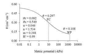
**Figure 2.** Soil water retention curve according to the van Genuchten model.  $\theta$ r: residual moisture,  $\theta$ s: saturation moisture, and  $\alpha$ , n, and m are tuning parameters. FC: field capacity and WP: wilting point.
