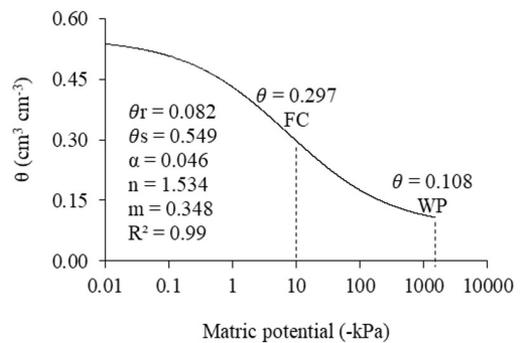
**Figure 2.** Soil water retention curve according to the van Genuchten model. θ<sub>r</sub>: residual moisture, θ<sub>s</sub>: saturation moisture, and α, n, and m are tuning parameters. FC: field capacity and WP: wilting point.
