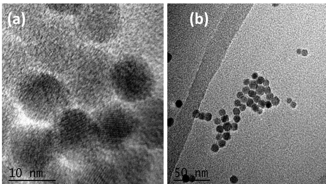
**Figure 1.** View of Selenium Nanospheres by Transmission Electron Microscopic (a) 10nm scale bar (b) 50nm scale bar with magnified form.
