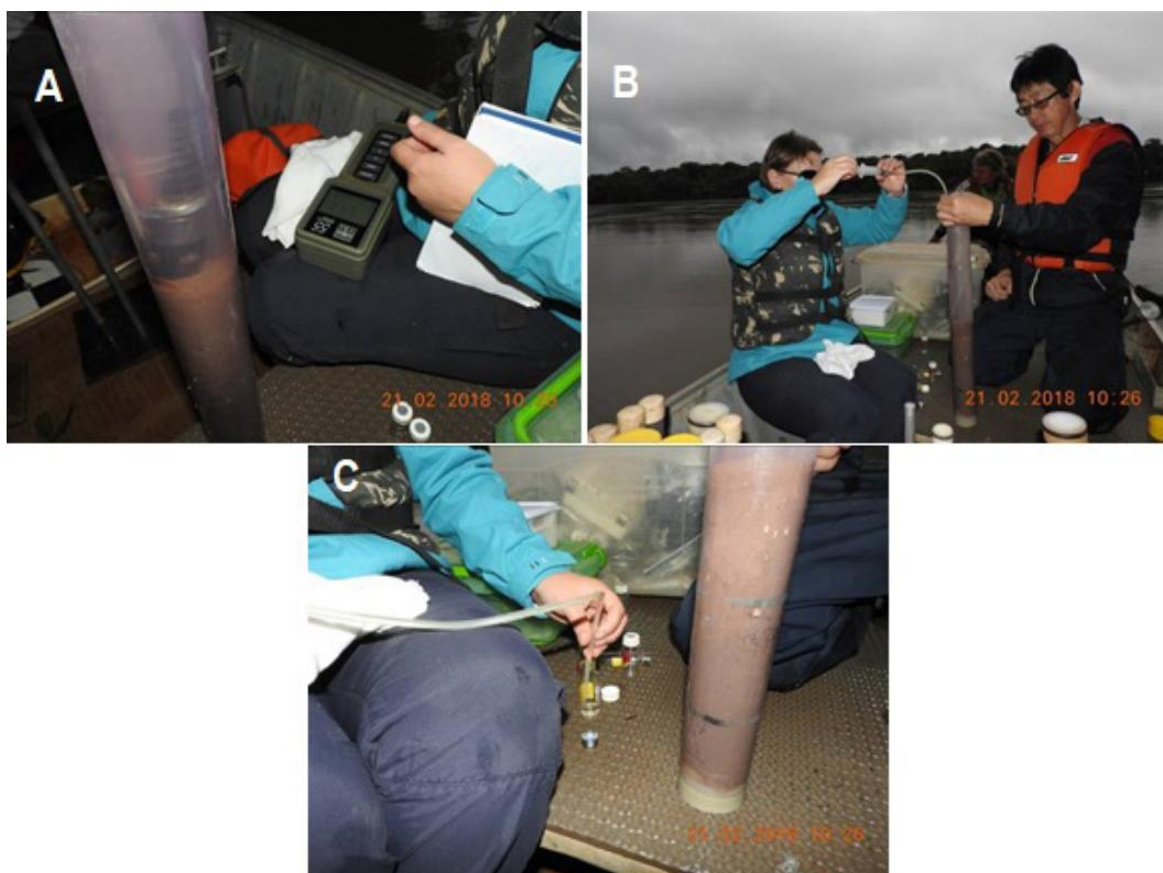
**Figure 4.** Photographic record of the quantification of temperature and dissolved oxygen (A) and the collection of water samples (B and C) for the quantification of  $\text{CO}_2$  in the layer above the sediment-water interface in the sediment core collected in the future reservoir of UHE Sinop. Source: AIIEGA (2018).
