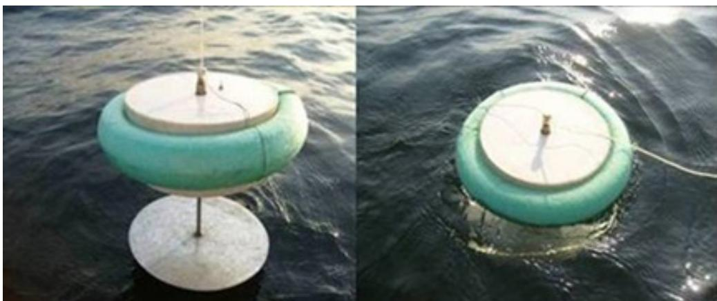
**Figure 2.** Diffusion gas collecting chamber showing protective shield against bubbles. Source: COPPE (2018).
