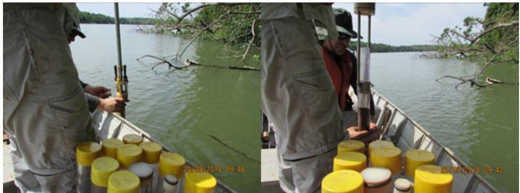
**Figure 3.** Photographic record of sediment sample collection in the future reservoir of HPP Sinop with the aid of a telescopic manual rod coupled to the Kajak-Brinkhurst type witness. Source: AIIEGA (2018).
