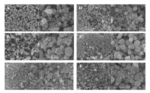
**Figure 2.** A. The SEM images of biosynthesized ZnO NPs (10-50 nm), B. SEM images of zinc oxide nanoparticles with little agglomeration C. Scanning electron microscopy images of zinc oxide nanoparticles for sample 3. D. SEM micrographs of zinc nanoparticles having size 50-100 nm. E. Micrographs of zinc oxide nanoparticles for sample 5. F. SEM images of ZnO nanoparticles (ZnO NPs in this case appears to be greater as compared to Figure 2E).
