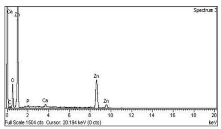
Figure 1. EDX spectra of zinc oxide nanoparticles.
