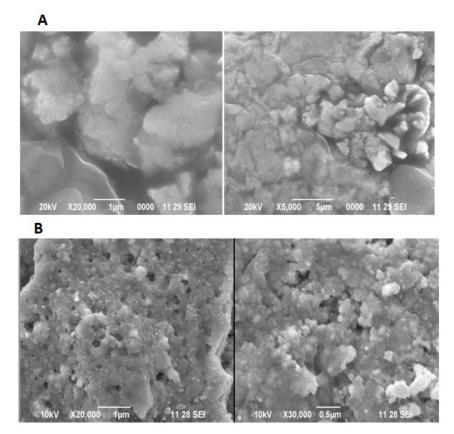
**Figure 3. A.** SEM images of silver nanoparticles synthesized using high concentration of *Passiflora foetida* extract. **B.** SEM images of silver nanoparticles synthesized using low concentration of *Passiflora foetida* extract.
