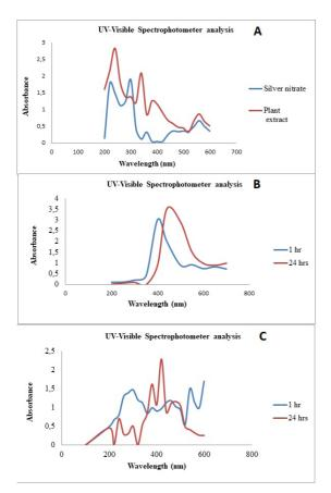
**Figure 1. A.** UV- Visible Spectroscopy Analysis of Silver nitrate and plant extract (Control). **B.** UV- Visible Spectroscopy Analysis of Silver nanoparticles synthesized using high concentration of plant extract. **C.** UV- Visible Spectroscopy Analysis of Silver nanoparticles synthesized using Low concentration of plant extract.
