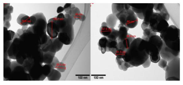
Figure 6. TEM images of silver nanoparticles synthesized using low concentration of Passiflora foetida extract.
