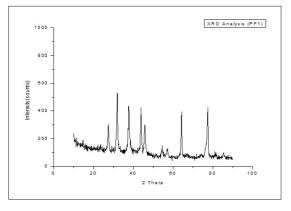
Figure 5. XRD Profile of silver nanoparticles synthesized using low concentration of *Passiflora foetida extract*.
