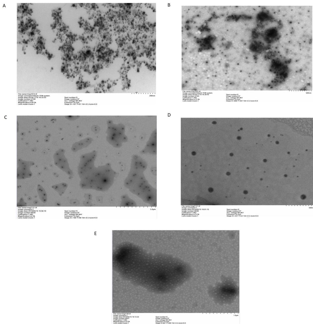
**Figure 7.** TEM results of Fusarium AgNP at pH 4 (A), at pH 5 (B), at pH 6 (C), at pH 7 (D) and without NP at pH 7 (E).
