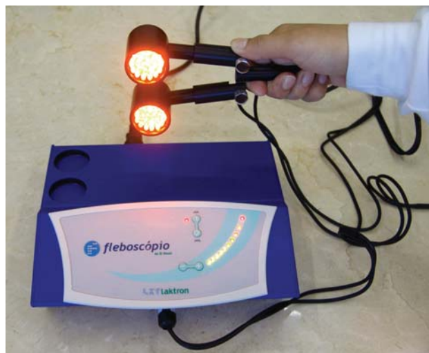
Figure 1 - Transillumination phleboscopia device
