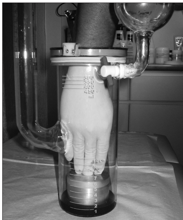
Figure 4 - Picture displaying the volumeter with communicating chambers in hermetic situation for collecting segmentary measures, sealed by the glove and edge-limiting rings and fastening rings, as well as the position in which the hand must be during volumetric reading
