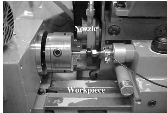
Figure 4. The cylindrical grinding process.
