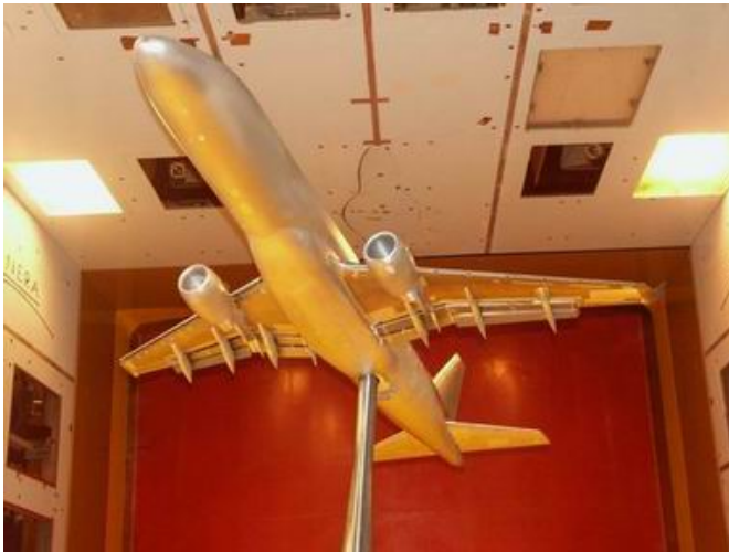
Figure 9. Subsonic pressurized tunnel test - EMBRAER 170 full model at ONERA F1.
