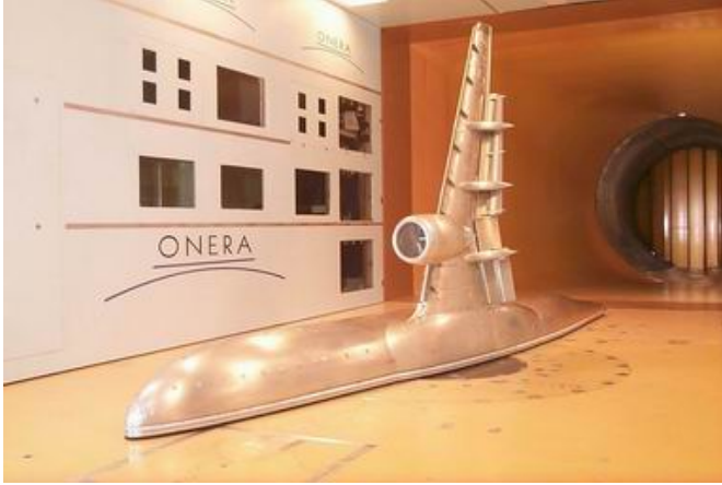
Figure 8. Subsonic pressurized tunnel test - EMBRAER 170 half model at ONERA F1.
