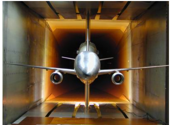
Figure 11. Transonic pressurized tunnel test - EMBRAER 170 at DNW/HST - Front View.
