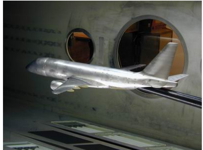
Figure 10. Transonic pressurized tunnel test - EMBRAER 170 at DNW/HST.
