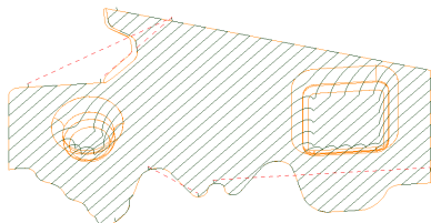
Figure 1. Zig-Zag cutting strategy with 45° cut direction.
