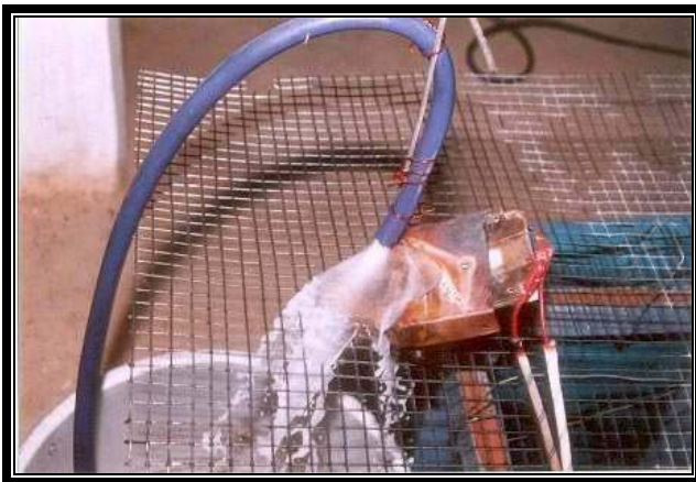
Figure 5. Pumping of fluids on the heated elements.
