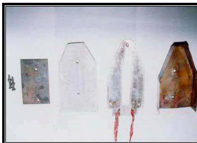
Figure 3. Individual components of heating element.
