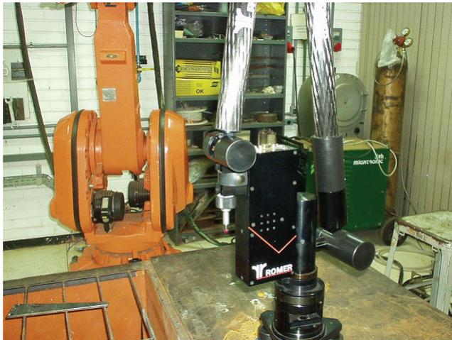
Figure 4. ITG ROMER measurement arm.
