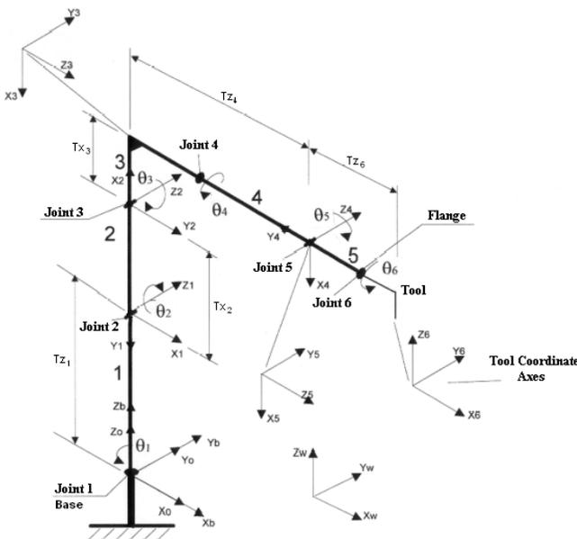
Figure 2. Kinematic Model of the IRB-2000 robot.
