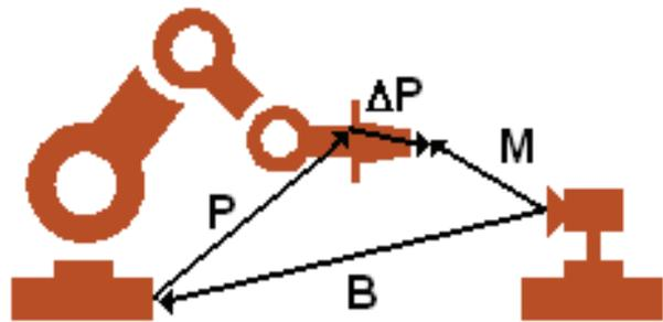
Figure 5. Calibration transformations.
