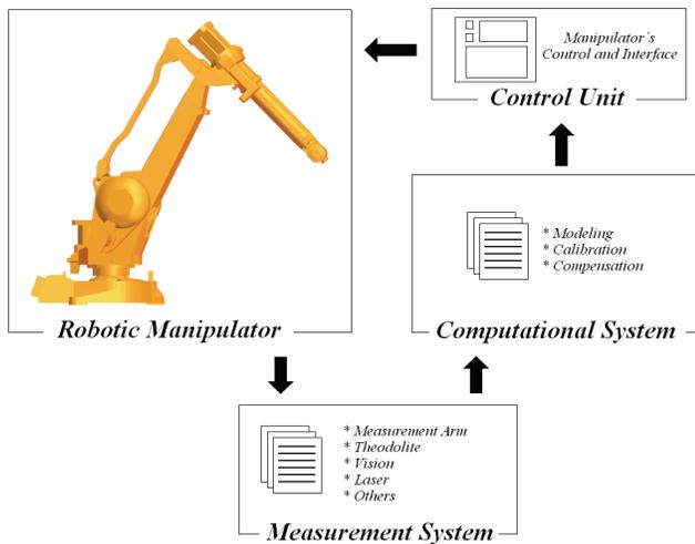
Figure 1. Block Diagram of the robot calibration system.
