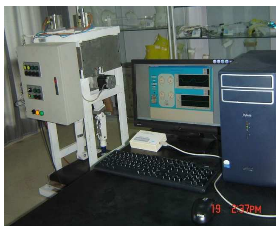
Figure 4. Simulation testing device for prosthetic leg.
