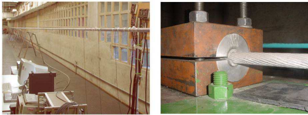
Figure 2. Photographs of the experimental set-up: (left) general overview of the CEPEL's laboratory span and (right) detailed view of conductor's clamp.
