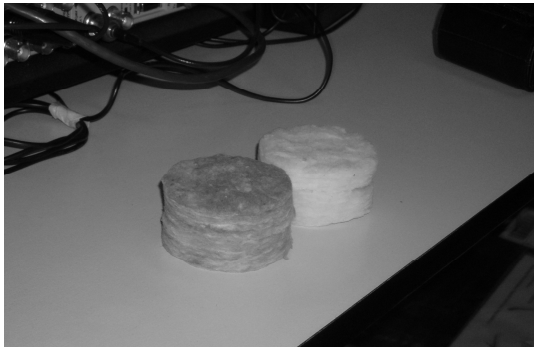
Figure 8b. Single-layered 0.42 pcf (light sample) and 1.0 pcf (dark sample), 3.0 cm thick each.
