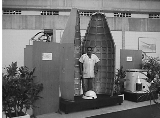
Figure 2b. VLS-1 fairing structure.
