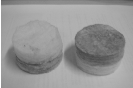
Figure 8a. Double-layered 0.42 pcf (light sample)/1.0 pcf (dark sample), 1.75 cm thick each.
