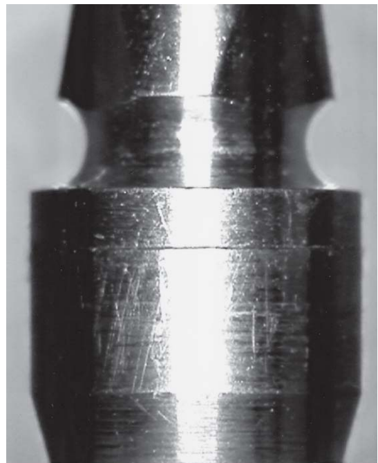
FIGURE 7- Marginal fit of pre-made metal cylinder at the abutment/cylinder interface
