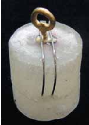
Figure 2- Custom cast dowel and core luted in a sample with simulated periodontal ligament. Note the presence of two wires in order to prevent the root dislodgement during testing
