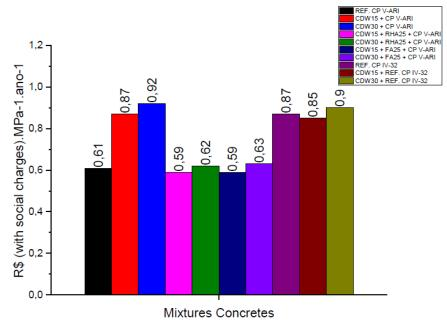
Figure 3 - Unit cost of different mixtures concrete
