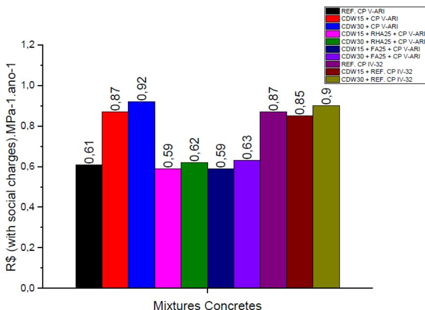
It can also be noted that the average unit cost was grouped by the strength class of concrete, with 0.88 R\$.MPa<sup>-1</sup>.year<sup>-1</sup> for concrete with fck = 25 years and 0.61 R\$.MPa<sup>-1</sup>.year<sup>-1</sup> for concrete with fck = 35 years, demonstrating the economic feasibility of binary concrete.
