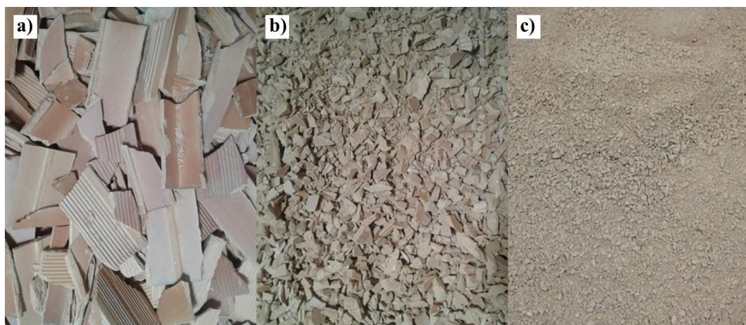
Figure 4 - Clay brick waste grinding evolution - (a) material collected, (b) after primary grinding and (c) after secondary grinding
