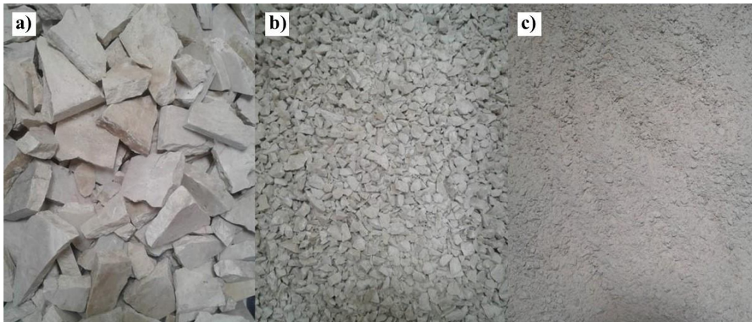
Figure 2 - Marble waste grinding evolution - (a) material collected, (b) after primary grinding and (c) after secondary grinding
