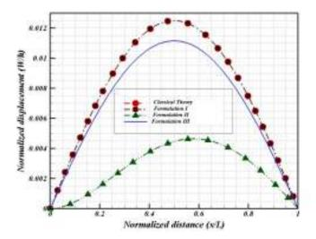
Figure 12: Normalized displacement of a simply-supported beam according to different theories with L=20h, b=2h, h=10g and g=0.02 nm.
