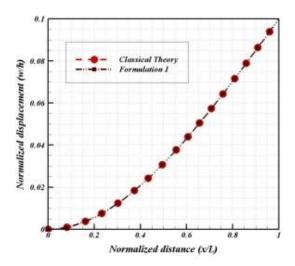
Figure 3: Normalized displacement of a cantilever beam according to the classical theory and formulation I with L=20h, b=2h, h=g and g=0.02 nm.
