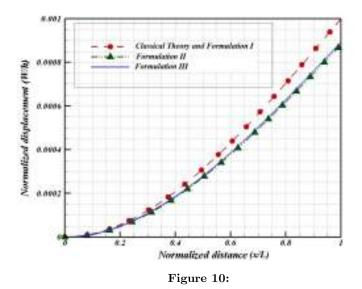
Figure 11: Normalized displacement of a cantilever beam according to different theories with L=20h, b=2h, h=10g and g=0.02 nm.
