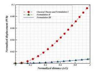
**Figure 7:** Normalized displacement of a cantilever beam according to different theories with L=20h, b=2h, h=g and g=0.02 nm.
