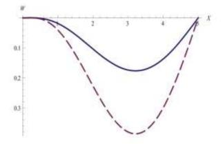
**Figure 5:** The elastic simply-supported micro-beam curve based on Lazopoulos and Lazopoulos (Lazopoulos and Lazopoulos, 2010) (solid line) and Papargyri-Beskou et al. (Papargyri-Beskou et al., 2003) (dashed line).
