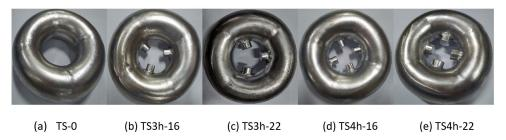
Figure 3 The test models of toroidal shell with openings; TS represents the toroidal shell, and 3h and 4h represent the openings number of toroidal shell, respectively. 16 and 22 represent the actual hole diameter of toroidal shells.
