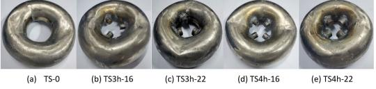
Figure 10. Toroidal shells with openings after failure.
