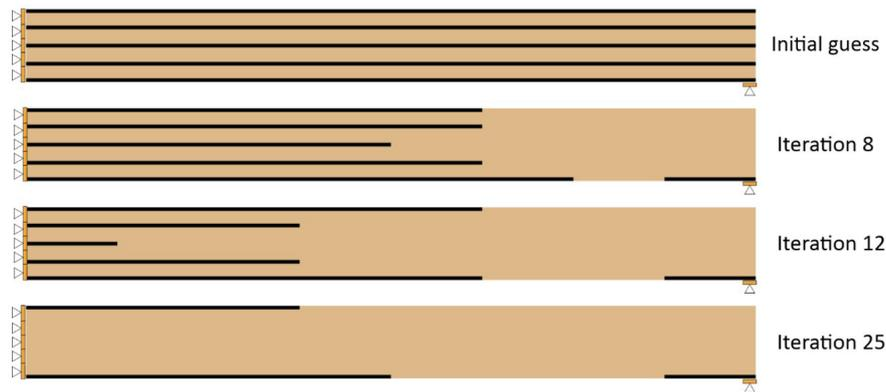
Figure 8 Four intermediate topologies with indication of the steel bars position from numerical example 1.
