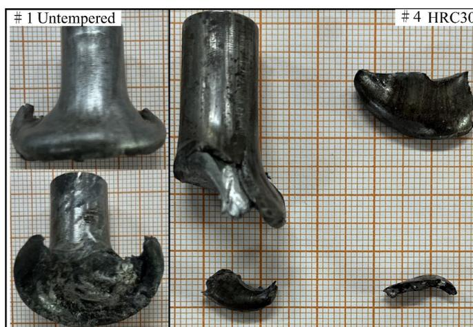
**Fig.7** PELE penetration behind target shape
