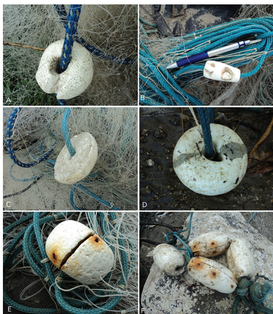
Figure 4. Damaged floats on net cables. A) Pressure marks showing wear of the cable on the float. B) Pufferfish bite marks. C) Float that was cut in half to reduce buoyancy. D) Floats that had been cut in half and then glued back together. E) Circular and F) cylindrical floats that were repaired using nails.
