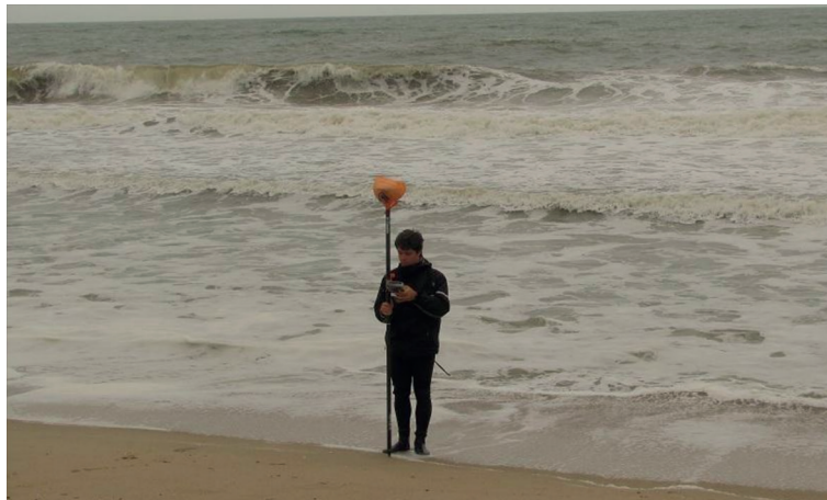
Figure 2. Maximum and instantaneous up-rush measurement on the beach face.
