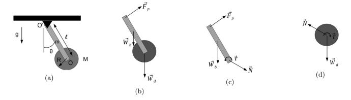
**Figure 1:** (a) Pendulum composed by a disk and a rod. (b) External forces acting on the rod-disk rigid system. In (c) and (d) the forces acting on the disk and rod are shown, respectively. The interaction between the disk and rod is represented by the force  $\vec{N}$  and the torque  $\vec{\tau}$ .
