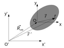
**Figure 3:**  $\vec{R}_{cm}$  and  $\vec{r}'$  represent the positions of the cm and of the point p relative to the inertial reference system O, respectively. Analogously,  $\vec{r}$  is the position of p relative to the cm.
