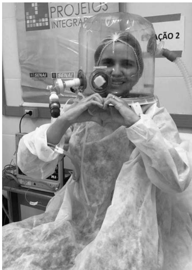
Figure 1. A physiotherapist wearing a prototype of a helmet-type system developed specifically for coping with COVID-19. The helmet allows the application of positive pressure around the head by means of a mixture of high flows of compressed air and oxygen, enabling an \text{FiO}_2 of up to 100% and continuous positive airway pressure of up to 18-20 \text{cmH}_2\text{O} , minimizing the risk of air leakage into the environment. Source: Personal archive of Holanda MA.
