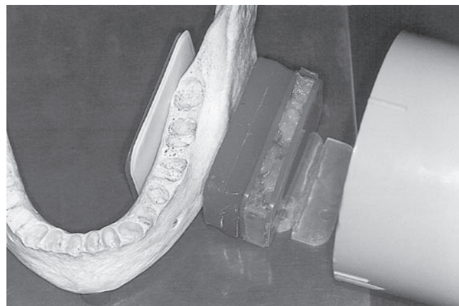
FIGURE 1 - Radiography taken with the set composed by radiographic film, mandible and simulators, parallel among each other.
