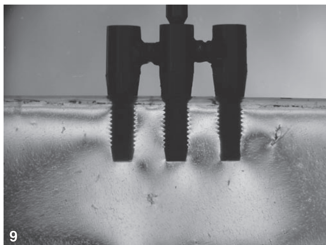
FIGURES 9 AND 10 - Photographic recordings of models P (9) and A (10), after the load application (5 kg).
