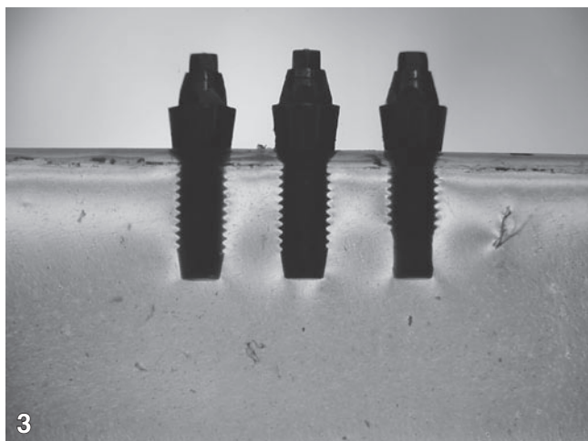
FIGURES 3 AND 4 - Photographic recordings of models P (3) and A (4), before the installation of the prosthesis and the load application.
