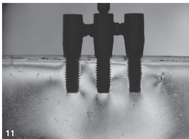
FIGURES 11 AND 12 - Photographic recordings of models P (11) and A (12), after the load application (10 kg).
