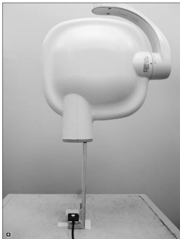
Figure 1 - (a) Sensor placed in the special device; X-ray tube aiming at the sensor; (b) Tooth slice positioned on the center of the sensor.
