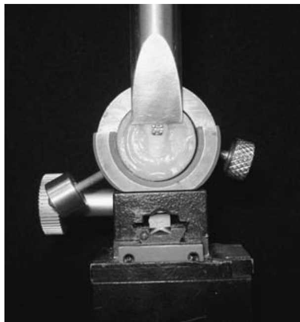
Figure 1 - Shear test by compression of a metal blade adapted to the mobile arm of the test machine.
