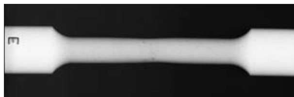
Figure 2 - Radiographic evidence of the presence of porosity in a 3.5-mm specimen with a 0.6-mm joint opening.
